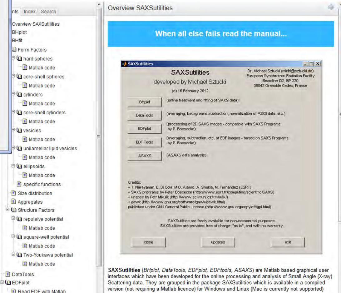
SAXSutilities (BHplot, DataTools, EDFplot, EDFtools, ASAXS) are Matlab based graphical user interfaces which have been developed for the online processing and analysis of Small Angle (X-ray) Scattering data. They are grouped in the package SAXSutilities which is available in a compiled version (not requiring a Matlab licence) for Windows and Linux (Mac is currently not supported)
