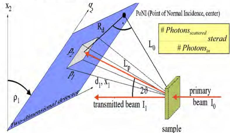
5. Normalization to transmission and scattering volume, e.g. thin film:
