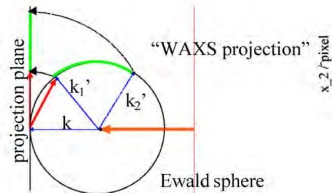
In Waxs projection the scattering pattern of a tilted detector can be geometrically analysed (azimuthal regrouping etc.) like a small angle scattering pattern.
