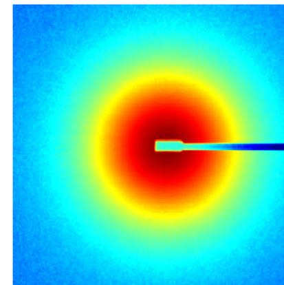
scattering of X-rays at small-angles originate from spatial fluctuations of the electron density within the material
